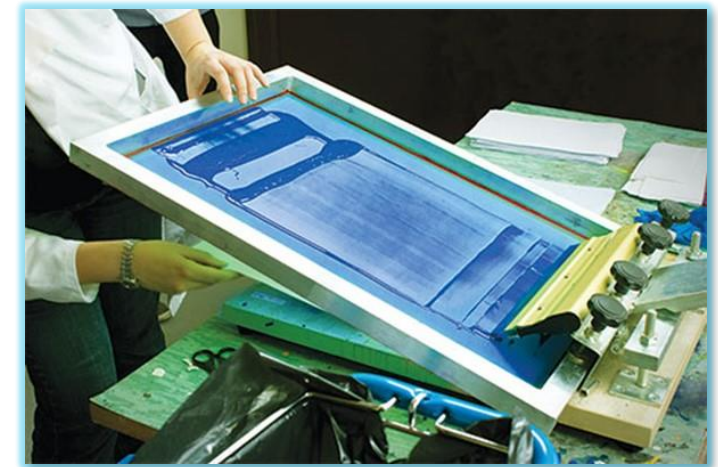
Metal frame printing screens with carriage
