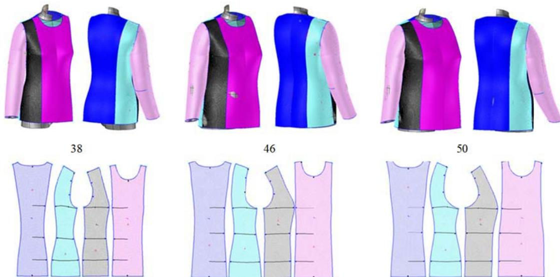
**Figure 10.** Top: Blouse construction in 3D size 38, morphological grading size 46, 50
