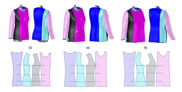
**Figure 10.** Top: Blouse construction in 3D size 38, morphological grading size 46, 50 Bottom: 2D pattern parts
