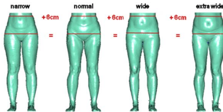
Fig. 2. Defining the waist types at constant hip circumference (e.g. hip circumference - 99 cm) [1].
