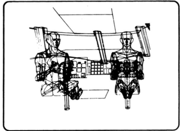
Figure 2. “First Man.” This seven-segment articulated pilot was used in studies of the Boeing 747 instrument panel (Boeing, 1968).
