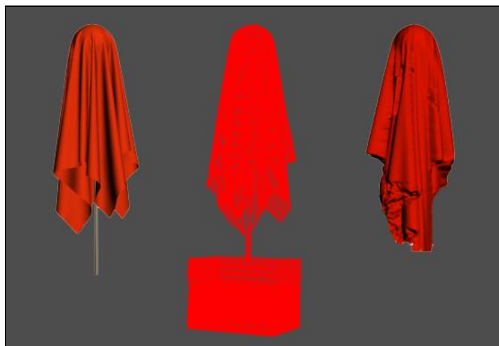
Figure 165: Comparison virtual simulation (left), scanned real fabric as point-cloud (center), scanned real fabric as polygons (right)
