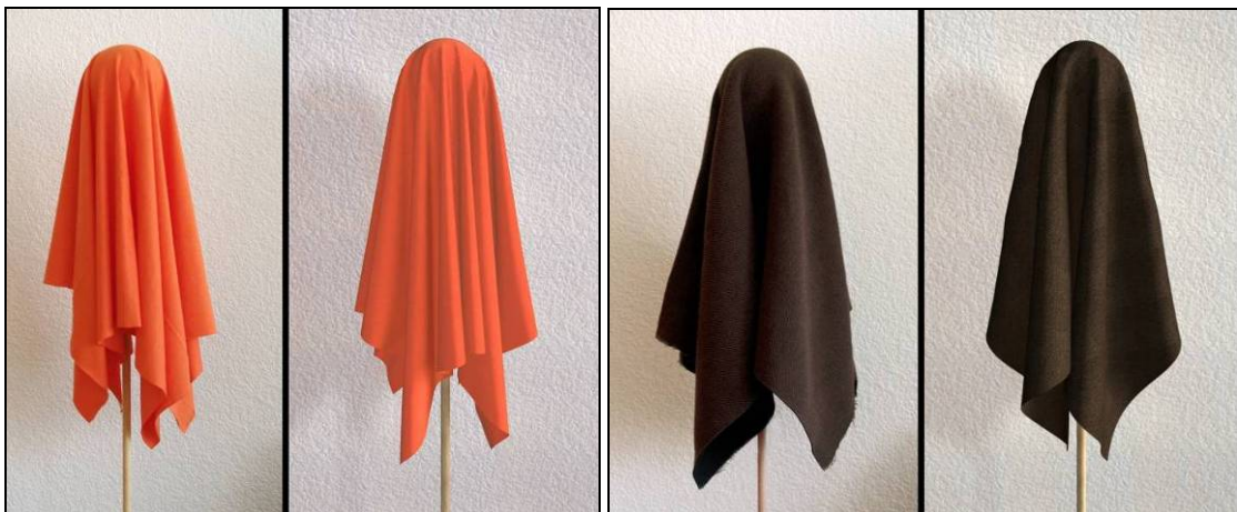
Figure 163: Fabric 38_single-jersey: real and virtual drape (left), fabric 36_overcoat fabric: real and virtual drape (right)
