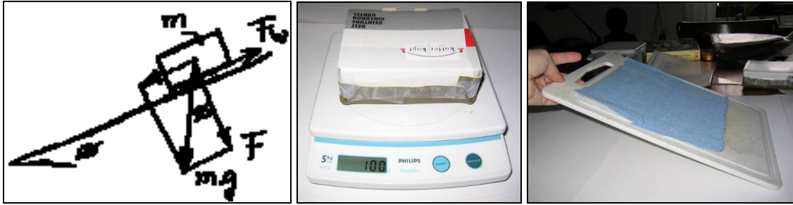
Figure 154: Scheme of friction evaluation [Tribol]
