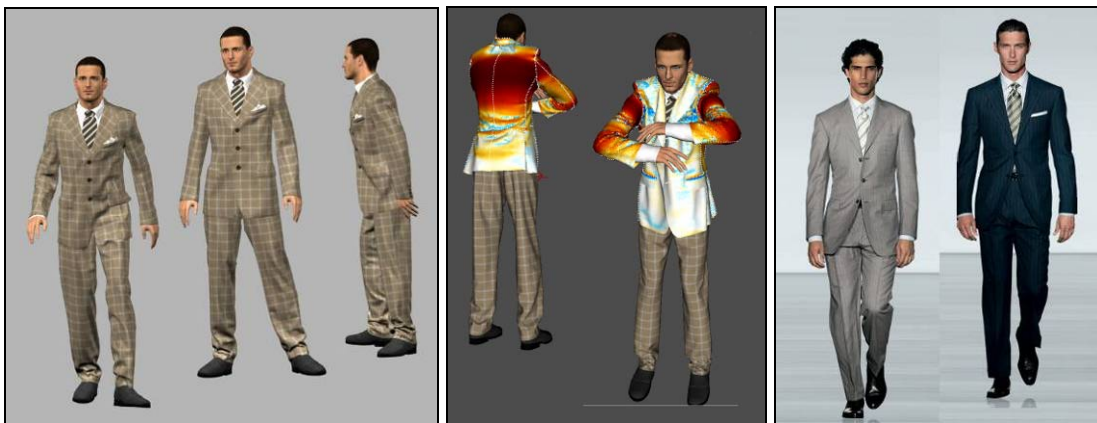
Figure 3: Virtual prototyping of men suits visualizing numerical fitting data (Miralab-University of Geneva), real men suits [Zegna]
