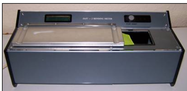
Figure 16: SiroFAST bending measurement machine [CSIRO 07]
