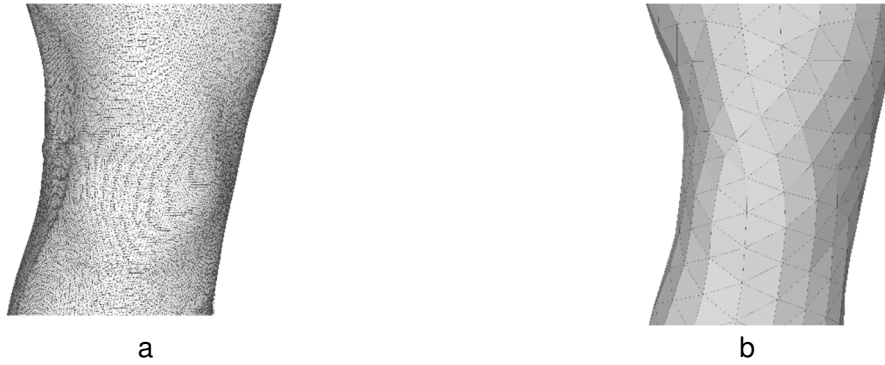
Fig.2. Reduction of triangle number, a) high-resolution scan; b) low-resolution triangle mesh.
