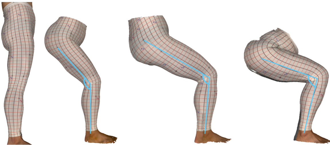
Fig. 1. Screenshots of 3D laser scan models of the leg in various poses (knee flexion angles of 180°, 136°, 114°, and 97°).
