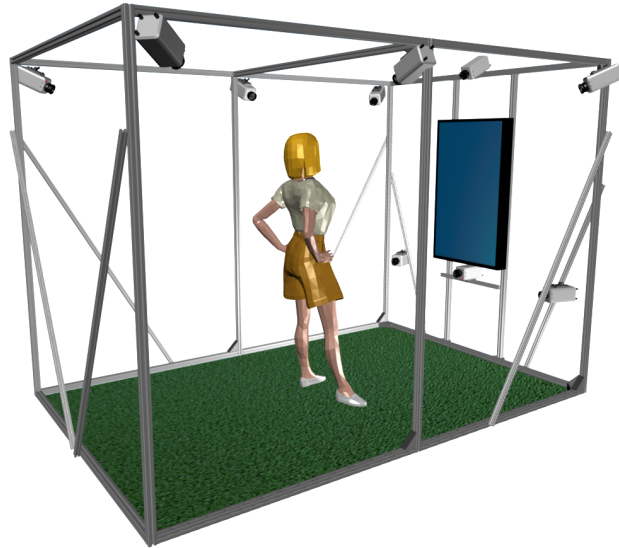
(a) Model of the recording setup with camera positions (without walls)
