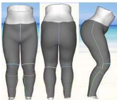
Figure 8: Virtual fit simulation of the obtained patterns for the tight-fitting trousers from 3D-to-2D technique
