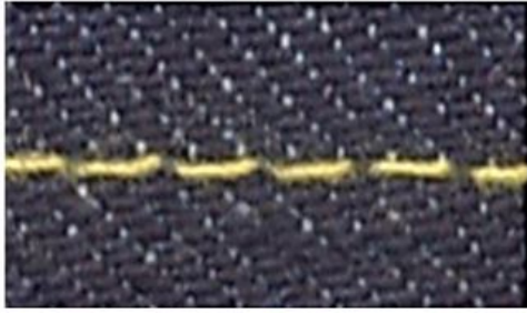
FIGURE 12. Appearance of the lockstitch on the surface of fabric type D3.
