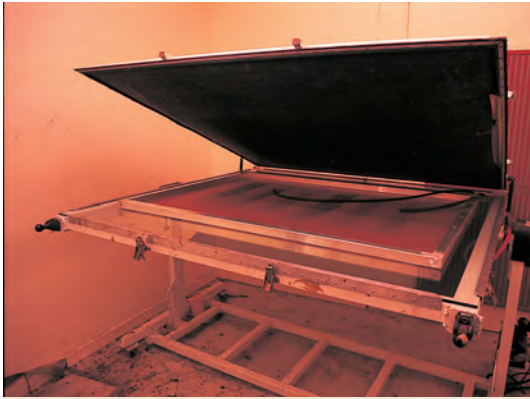
A vacuum frame is used in conjunction with a UV light source housed in a separate unit to expose screens at Double Helix's studio.
