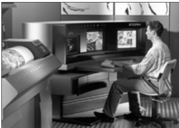
Figure 2.16 Drum-type colour scanner interfaced to CAD system (Stork Screens BV)
