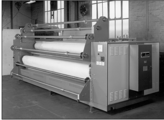
Figure 3.6 Rollingstatic MVZ 986, 3200 mm working width transfer-printing machine (Lemaire)
