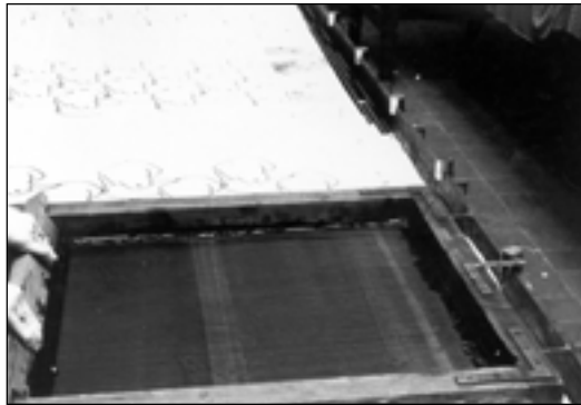
Figure 2.1 Hand screen printing showing stops, rail and bracket
