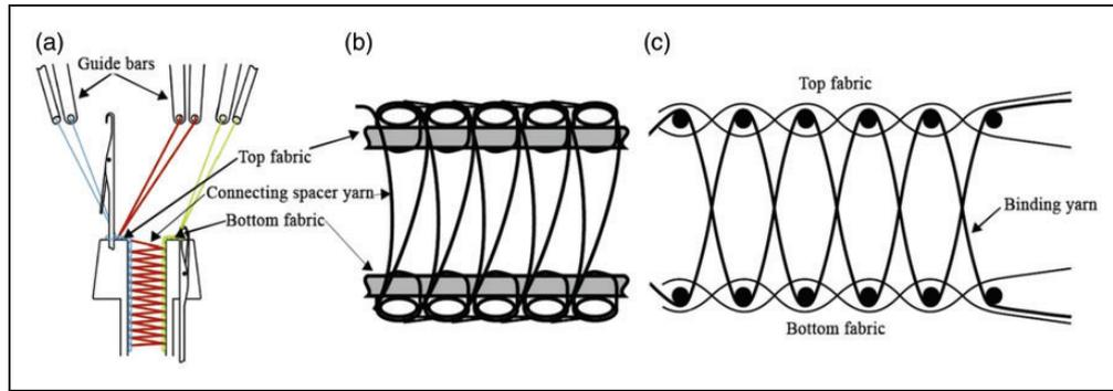
**Figure 5.** (a) Schematic of a double needle bar warp knitting machine. (b) Cross-section of a three-dimensional knitted spacer. (c) Cross-section of a woven double cloth (adapted from Wulffhorst et al.<sup>75</sup>).
