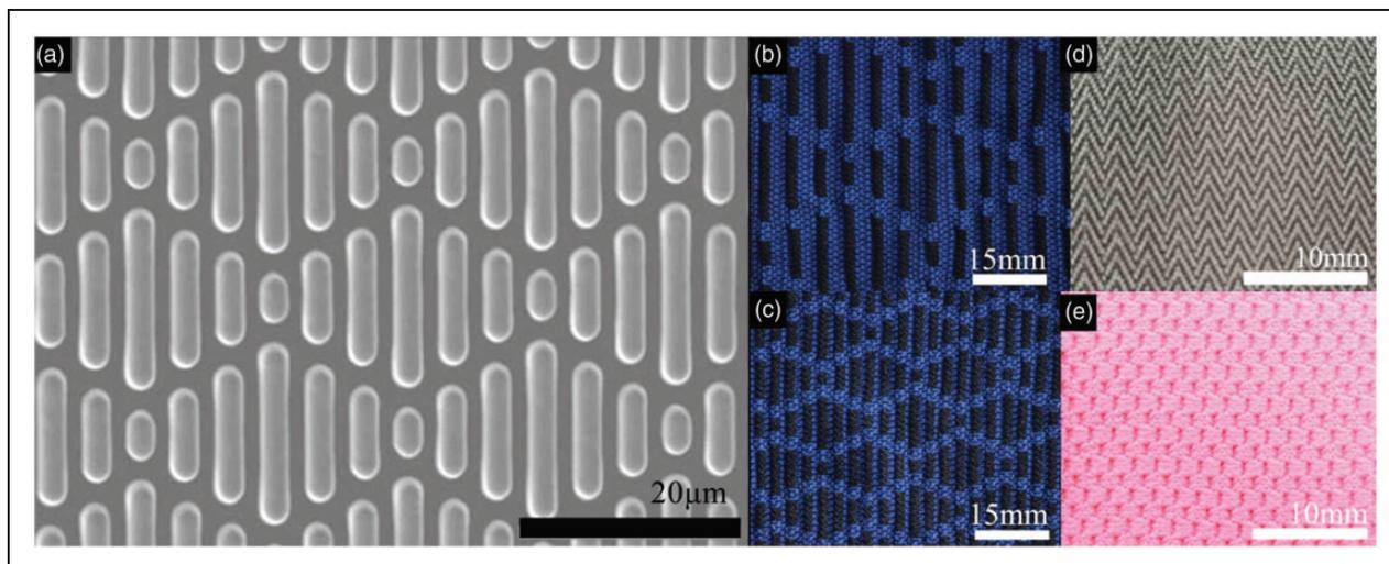
**Figure 4.** (a) Scanning electron microscopy image of Sharklet AF topography molded in Polydimethylsiloxane (adapted from Callow and Callow<sup>73</sup>). (b), (c) Knitted fabrics following the three-dimensional (3D) microstructured pattern of (a). Commonly found (d) knitted and (e) woven fabrics with comparable 3D structures to (a).
