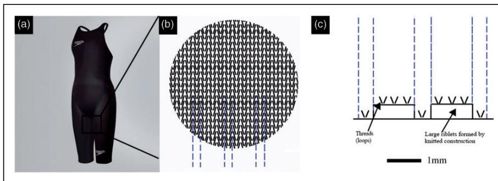
**Figure 2.** Speedo FastSkin<sup>®</sup> swimsuit and (b) stretched swimsuit close up. (c) Schematic showing apparent hierarchical riblet structure formed by threads (adapted from Bhushan<sup>64</sup>).
