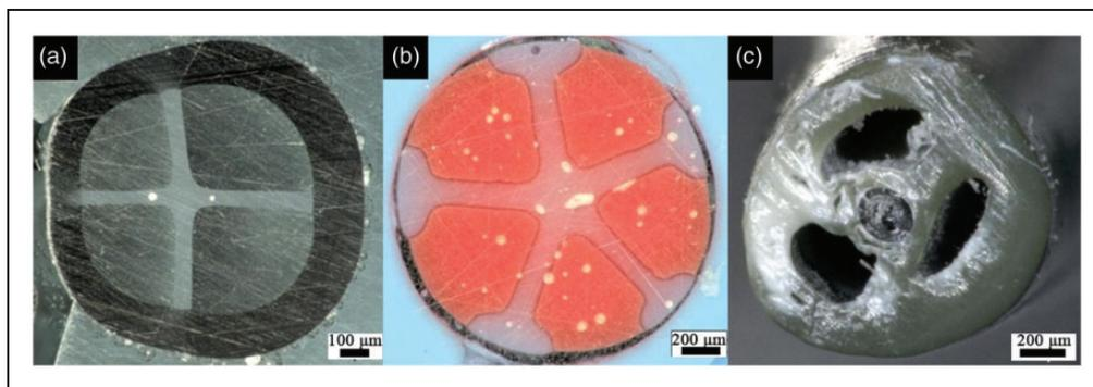
**Figure 6.** Microstructured monofilaments produced by heat drawing additive manufactured polymer preforms (adapted from Toal et al.<sup>76</sup>).
