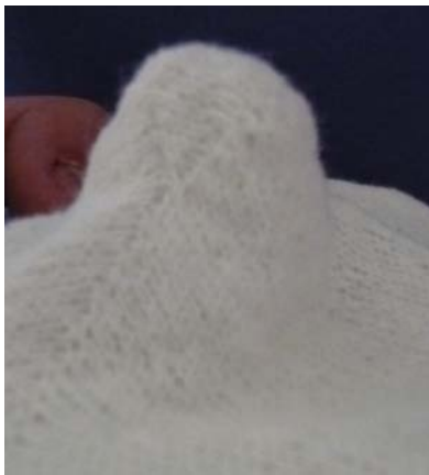
Figure 5: Spatial fashioned fabric – fabric aspect and knitting programme
