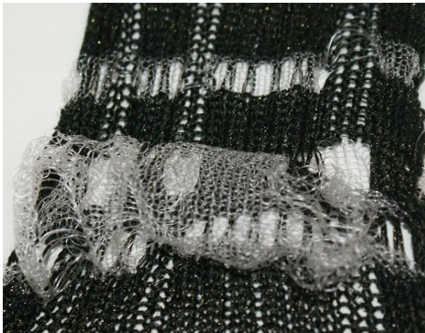
Figure 30: Ripple on the lace structure of composite structure and material knit (Yun, 2014).
