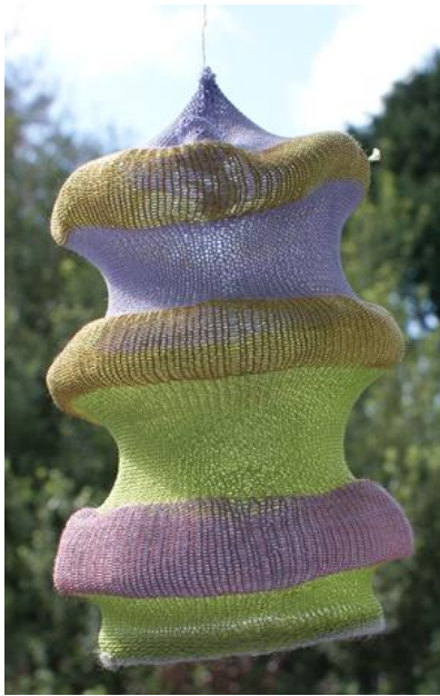
Figure 38: Thin cotton and composite 0.12mm copper stripes, knitted on 8 gauge hand-flat (Yun, 2014).
