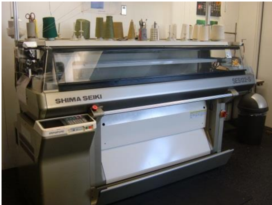
Figure 71: Shima Seiki SES122-S, 8 gauge (Yun, 2014).
