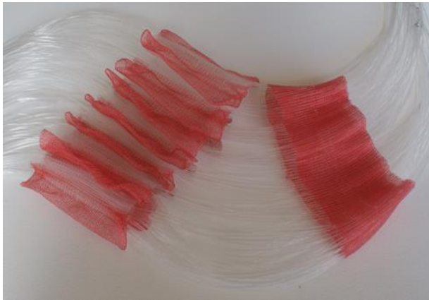
Figure 26: Fibre optic strands inserted through a 3D ripple structured copper composite on the left and a separate double knit copper composite piece on the right (Yun, 2014).
