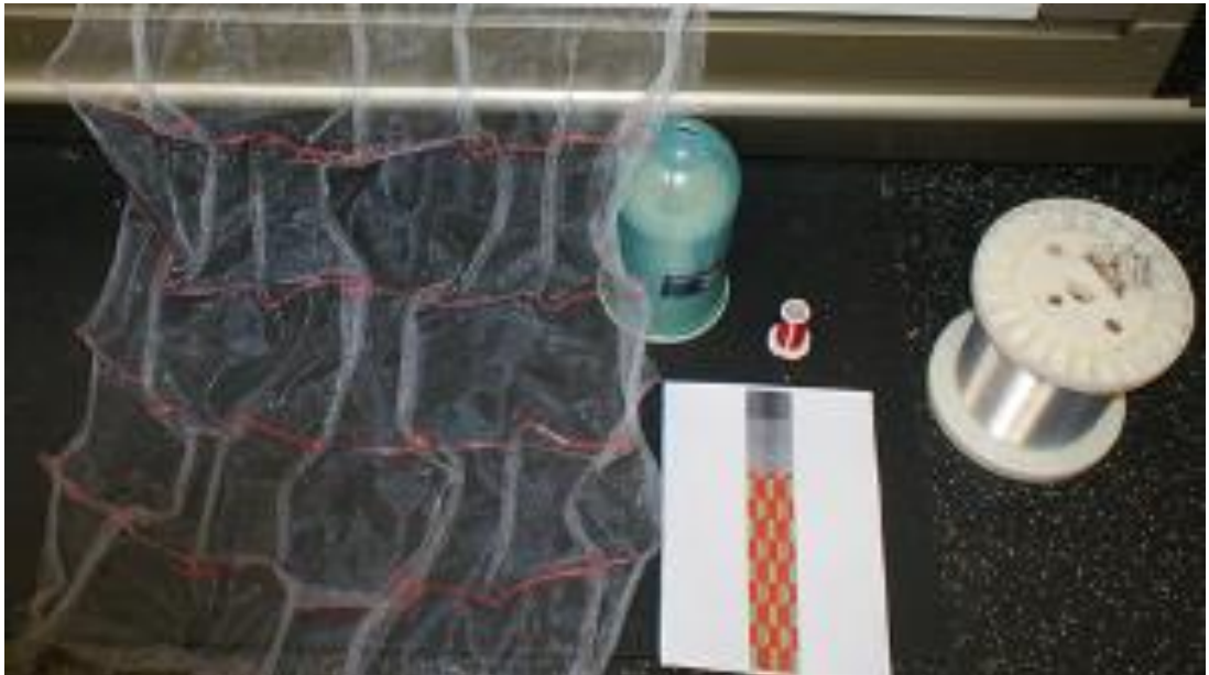
Figure 24: Placing spools of monofilament and copper on the floor can help avoid kinks and tangles when knitting (Yun, 2014).
