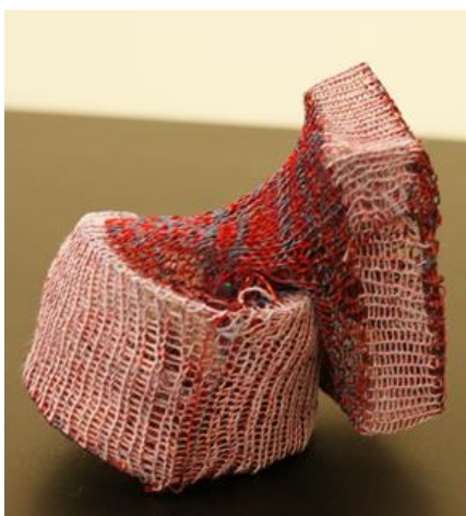
Figure 40: 0.3mm copper and cotton, knitted on 3 gauge hand-flat (Yun, 2014).
