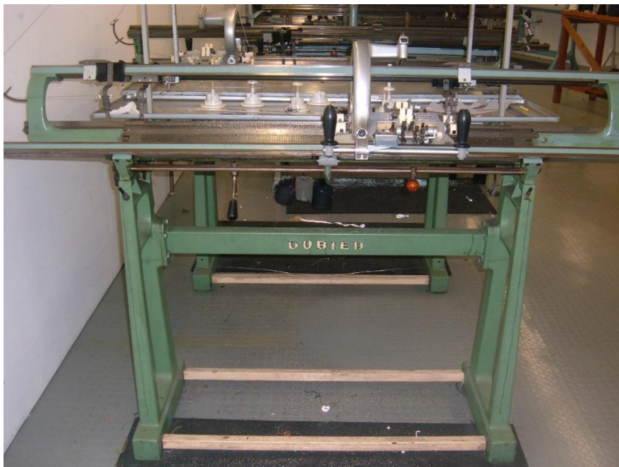
Figure 72: Dubied hand-flat knitting machine, 8 gauge (Yun, 2014).
