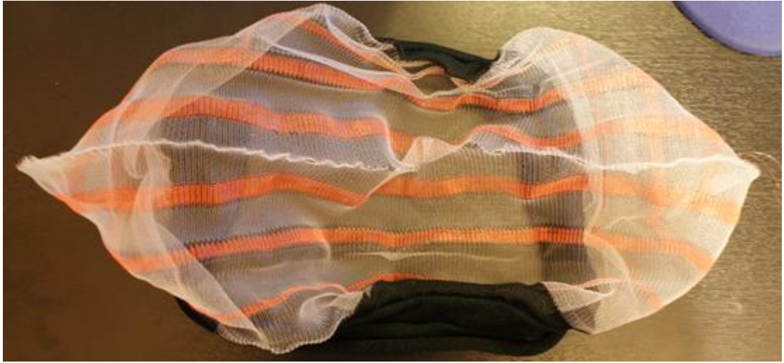
Figure 23: Plain copper stripes knitted on the Shima Seiki SES122-S (Yun, 2014).
