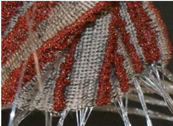
Figure 32: Copper and monofilament ripples (red) between monofilament and acrylic double knit (flecked grey) containing interlaid fibre optic strands (straight white strands), knitted on a hand-flat (Yun, 2014).
