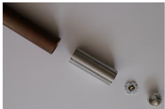
Figure 58: Actual prototype light showing aluminium heat sink second from left (Yun, 2014).
