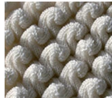
Figure 7: An example of a "Links-links" 3D surface knit fabric (Underwood, 2009, p. 79).
