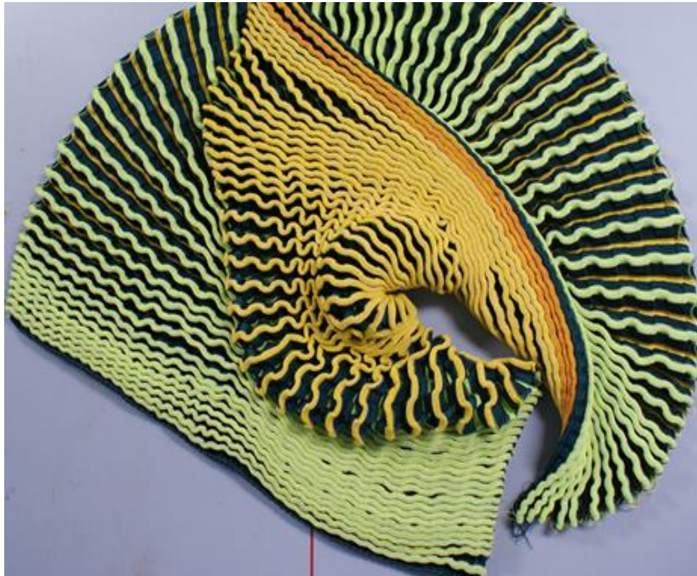
Figure 93: Test display of 3D surface knit (UV reactive acrylic and cotton) (Yun, 2014).
