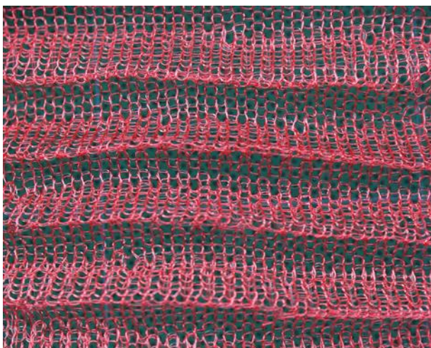
Figure 31: This series of small ripples were knitted on the SES122-S using copper and monofilament (Yun, 2014).
