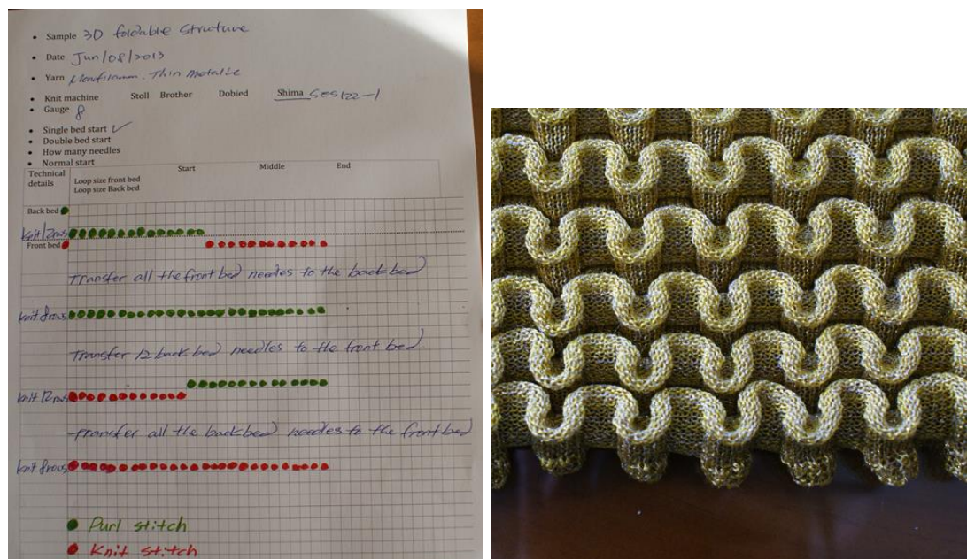
Figure 80: Knit notation template with foldable knit structure pattern (left) and sample of this fabric (right) (Yun, 2014).
