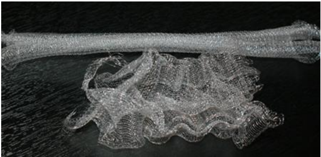
Figure 22: Plain stitch or ‘Jersey stitch’ of single knit on the top and 3D structure knit on the bottom (Yun, 2014).
