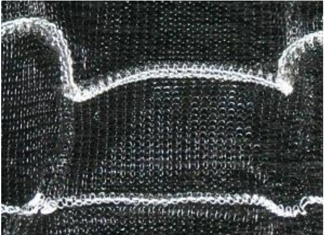
Figure 25: Monofilament knit with 4 rows of 0.3mm wide retro-reflective ribbon (and monofilament) at top and 2 rows below (knit on the Shima Seiki SES122-S) (Yun, 2014).
