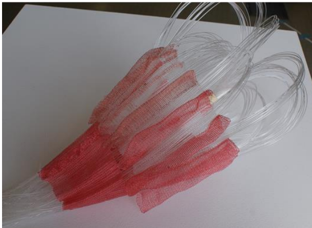
Figure 27: Twisting bottom of the fiber optic bundle to put inside of the fabric for a shaping (Yun, 2014).
