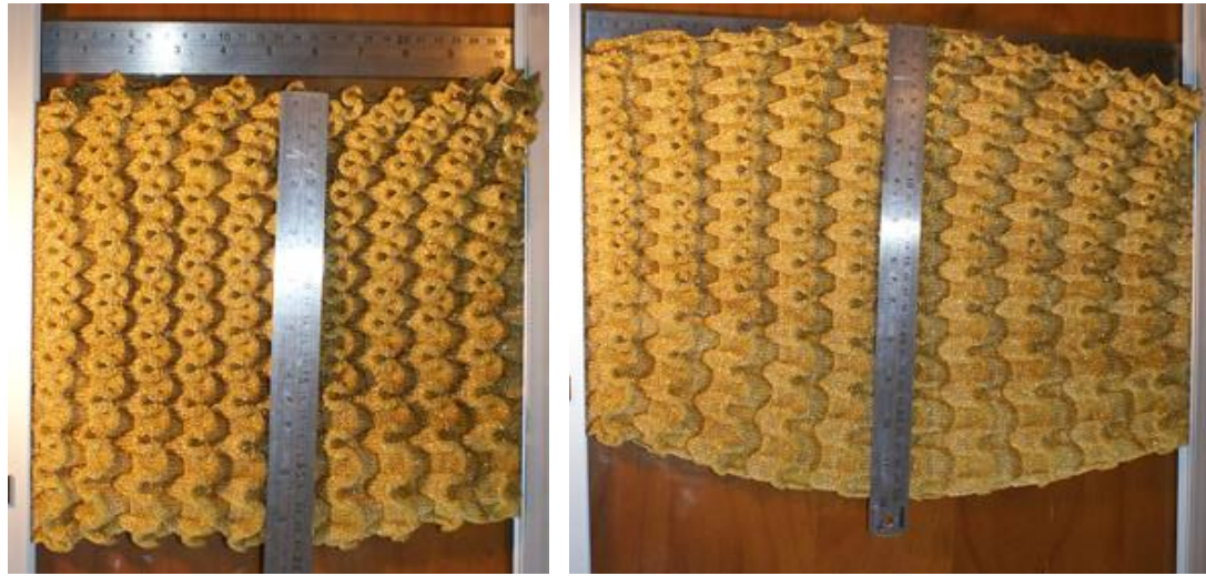
Figure 81: Monofilament and ‘metal sparkle’ acrylic 3D folding surface fabric. Unstretched left, Stretched right (Yun, 2014).
