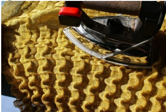
Figure 85: Hot iron test (Yun, 2014).
